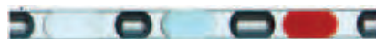
Figure 1. An array of differently colored aqueous samples separated by air bubbles (dark segments) in a capillary filled with a fluorocarbon.
