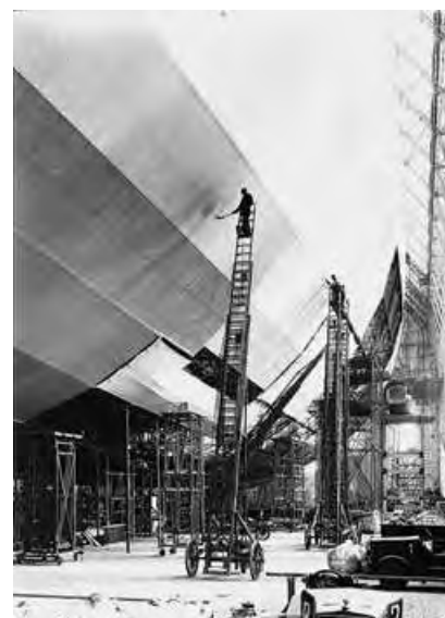
Figure 6. Multiple "Cellonization" of the external surface of a zeppelin made it impervious to gases and weather resistant, as well as conferring upon it streamlining characteristics. Photo: Archiv für Luftschiffbau Zeppelin GmbH, Friedrichshafen.
