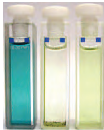
Figure 2. Color and solubility of zinc chlorin 6b in THF (left) and in heptane with 1% THF after 8 days (right) compared to that of model compound 1 (middle, also in heptane with 1% THF after 8 days).
