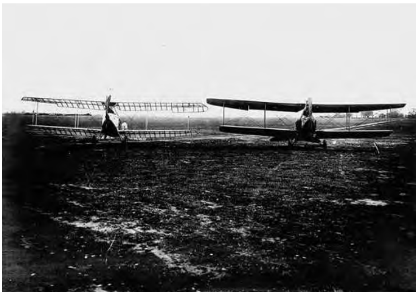
Figure 7. A nearly invisible military aircraft with a Cellon covering, together with a plane covered as usual with cloth. The “transparent airplane characterized by a weather-resistant covering consisting of roughly 1/10 cellulose derivative and 9/10 camphor substitute and gelatinizing agent” was patented during World War I, but remained an object of technical utopia. Photo: Bayer-Archiv, Leverkusen.
