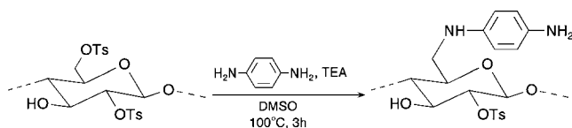
Scheme 11. Synthesis of PDA-cellulose by reaction of cellulose tosylate with 1,4-phenylenediamine (PDA).
